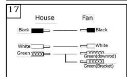
Make wire connections as per above diagram. Connect the white wire from the fan to the White or Neutral wire from the power source. Connect the black wire from the fan to the Black or hot wire from the power source. Connect all Green / Yellow wires from the fan, Downrod and mounting bracket to the Ground wire from the house.
